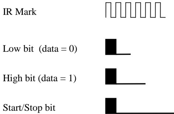
The high pulse illustrates six 38 kHz cycles.
