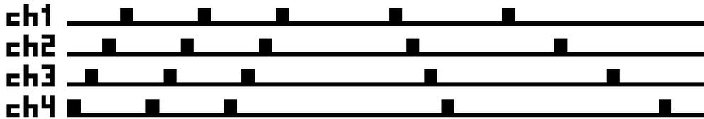
When a button is held down and the protocol needs update to prevent timeout the message is send continuously with a time interval as between message 4 and 5. First after all buttons are released and this is transmitted the transmitter will shut down.
