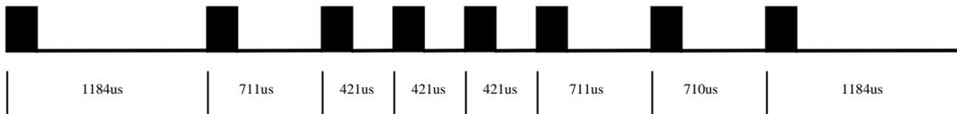
When the stop bits pause is reached the message is processed.
